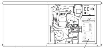
Fuel Pump & Fuel Filter / (Behind Access Panel & Air Filter)
